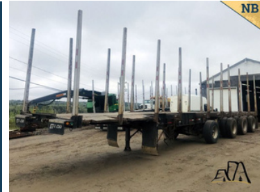
2017 BWS 51' Q/A Log Trailer Air ride, steerable axle, plumbed for self loader. Asking $45,000
