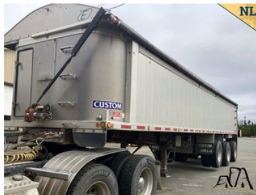
2018 Custom End Dump Trailer 37' box, air ride, 2 lift axles, electric tarp, teflon liner. Asking $75,000
