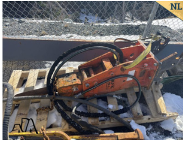
NPK PH-3 Hydraulic Hammer To fit Deere 50G. 500 hours. $35,000
