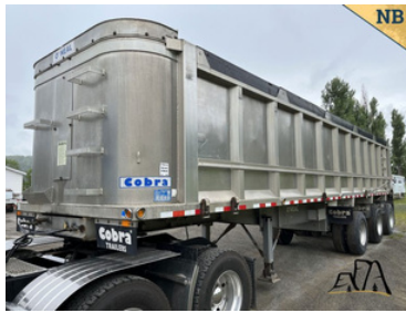
2004 Cobra End Dump Trailer Tri axle, 37' aluminum body, air ride, teflon liner. Asking $50,000
